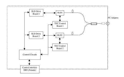
Figure 1 Configuration of IPSDW0825-xxxx SLD light source module
