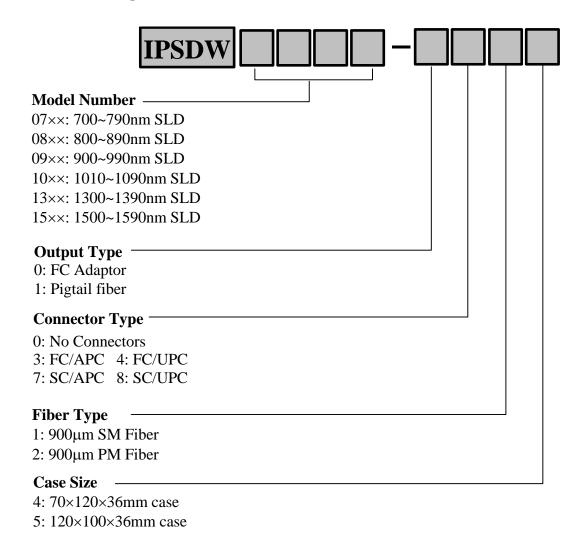
**Example**: IPSDW0821-0314: 800nm-type SLD module in 70×120×36mm case with FC adaptor output, FC/APC connector and 900μm SM Fiber.
