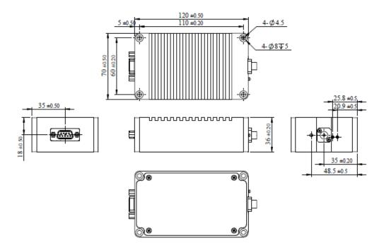
Figure 2 Mechanical drawing of IPSDW0825-0314 module
