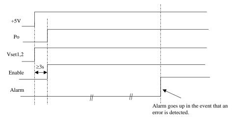
Figure 3 Startup and operational timing of IPSDW0825 module
